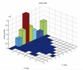
The tall columns represent the large number of low amplitude cycles, whereas the more extreme loads occur fewer times the shallow "tiles" to the right hand side.
