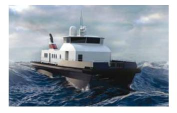
Due to be launched at the end of 2012 the SeaStrider SWATH (Small Waterplane Area Twin Hull) project from Danish Yachts is an innovative solution for crew transport vessels.
